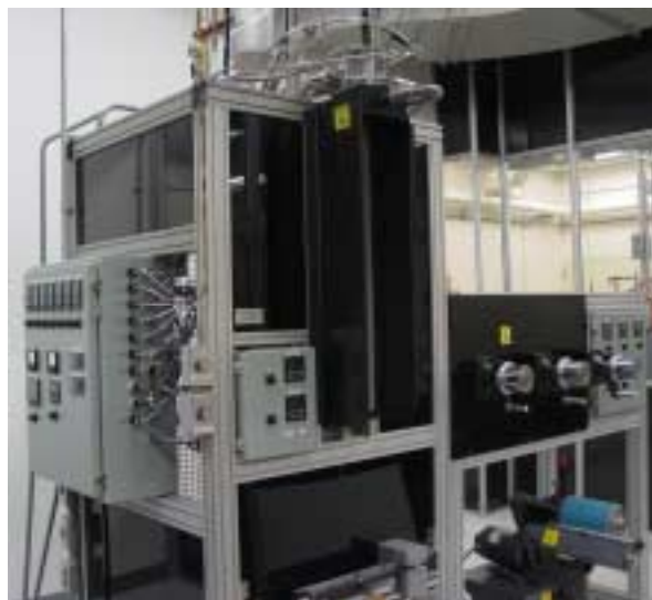
Figure 6. New melt-spinning equipment.
